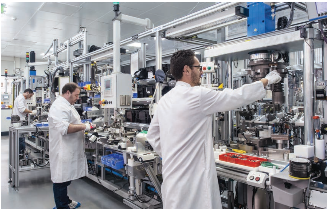
Liebherr Machines Bulle has plans to roll out the lean management approach across the company. The first to receive the lean treatment is its production unit. Here, the diesel injection system assembly line in the LMB clean room.
