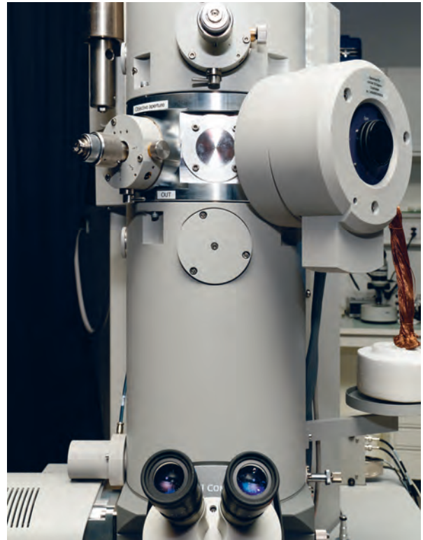
The AMI's Transmission Electron Microscope (TEM) detects nanoparticles using a high-voltage electron beam.
