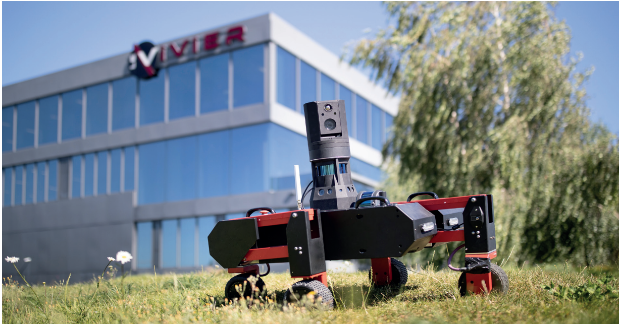
Thanks to its on-board battery, the 50 kg, one-meter-long ROVéo can run for eight hours non-stop.
