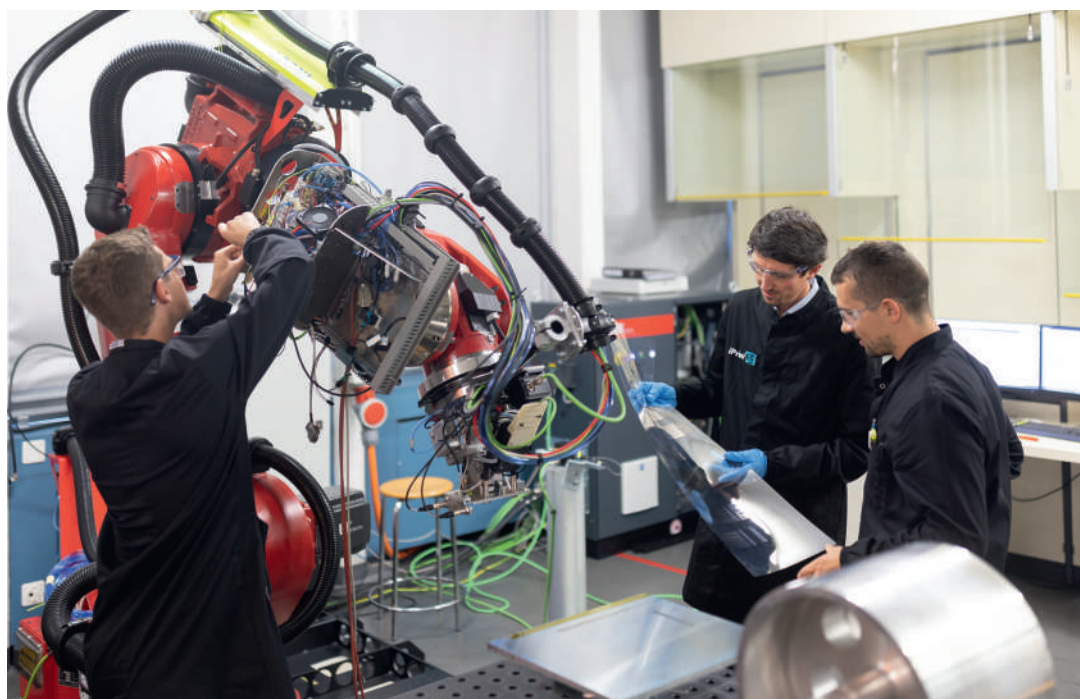
'Direct-to-shape (DTS)' is the name of iPrint's joint project with two companies, Polytipe and MABI Robotic. The trio aims to develop a more effective robotics-based method of printing directly on to large 3D objects.
